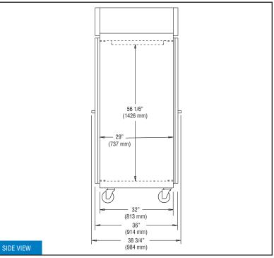
**IMPORTANT NOTE:** If the cabinet is located under a low ceiling, a <u>minimum clearance of 12" is required on</u> top and 3" on sides.
