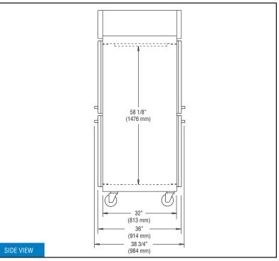
**IMPORTANT NOTE:** If the cabinet is located under a low ceiling, a <u>minimum clearance of 12</u>" is required on top and 3" on sides.
