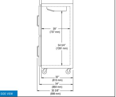
IMPORTANT NOTE: If the cabinet is located directly against a wall and/or under a low ceiling, a minimum clearance of 12" is required on top and 3" on sides and rear.
