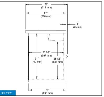
**IMPORTANT NOTE**: Models are completely front breathing and take in and exhaust air through the front grill. For proper operation, the area in front of the cabinet **must** not be obstructed in any way. A clearance of 1" on the back and 3" on the sides is recommended.
