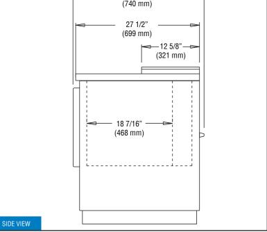
**IMPORTANT NOTE:** Model is completely front breathing and takes in and exhausts air through the front grill. A clearance of 1" on the back and 3" on the sides is recommended.
