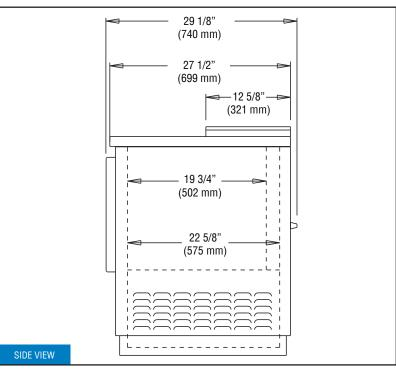
**IMPORTANT NOTE**: A <u>minimum clearance of 3" is required</u> on each side, front and rear of cabinet for optimum performance.
