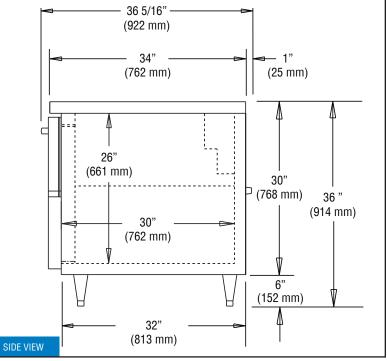
**IMPORTANT NOTE:** If the cabinet is located directly against a wall, a <u>minimum clearance of 3" is required</u> on sides, front and rear.
