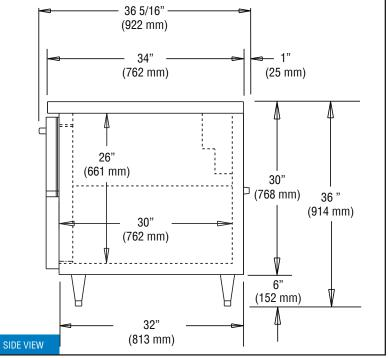
**IMPORTANT NOTE:** If the cabinet is located directly against a wall, a <u>minimum clearance of 3" is required</u> on sides, front and rear.
