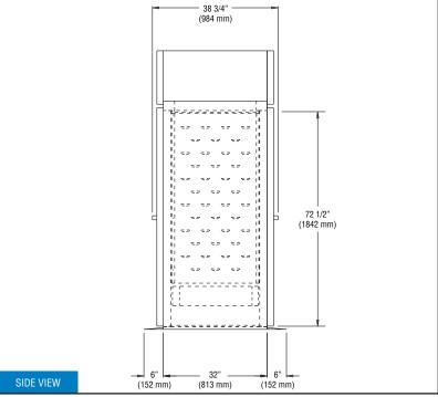
IMPORTANT NOTE: If the cabinet is located directly against a wall and/or under a low ceiling, a minimum clearance of 12" is required on top and 3" on sides.
