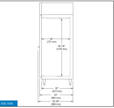
IMPORTANT NOTE: If the cabinet is located directly against a wall and/or under a low ceiling, a minimum clearance of 12" is required on top and 3" on sides and rear.
