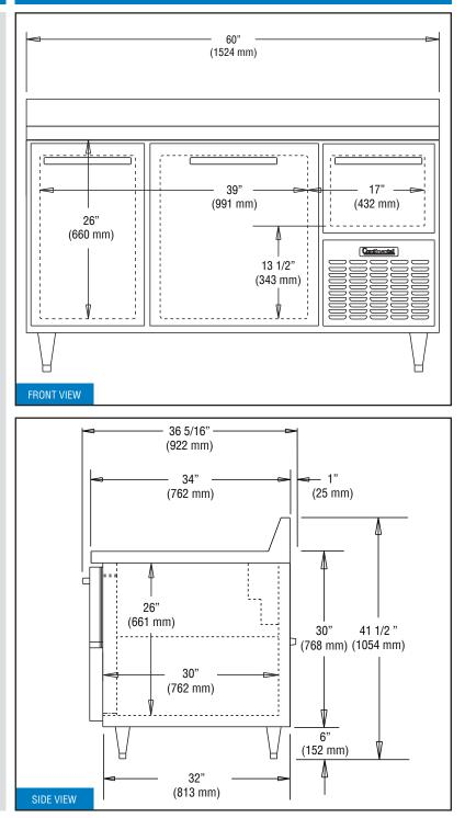
**IMPORTANT NOTE:** If the cabinet is located directly against a wall, a <u>minimum clearance of 3" is required</u> on sides, front and rear.
