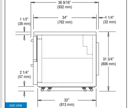
NOTE: For proper operation, the area under and in front of the cabinet must not be obstructed in any way.
