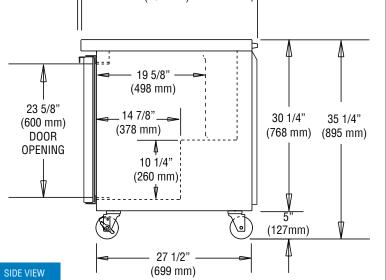
IMPORTANT NOTE: If the cabinet is located directly against a wall, a minimum clearance of 3" is required
