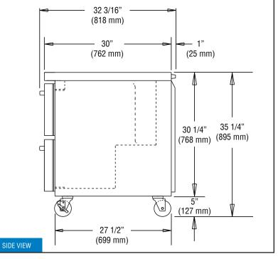
IMPORTANT NOTE: If the cabinet is located directly against a wall, a minimum clearance of 3" is required on sides, front and rear.
