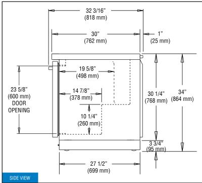
$\underline{\textbf{NOTE}}\text{: For proper operation, the area under and in front of the cabinet }\underline{\textbf{must}}\text{ not be obstructed in any way.}$
