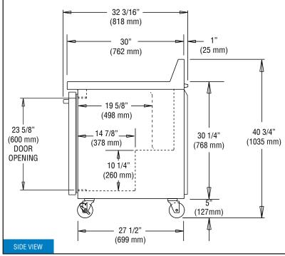
**IMPORTANT NOTE:** If the cabinet is located directly against a wall, a <u>minimum clearance of 3" is required on sides, front and rear.</u>
