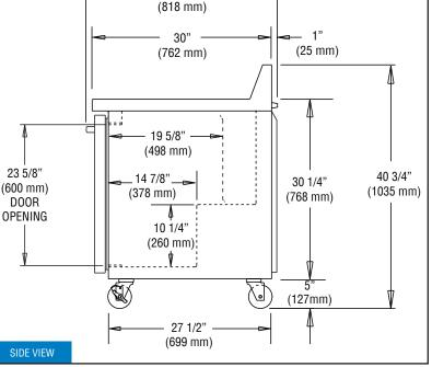
**IMPORTANT NOTE:** If the cabinet is located directly against a wall, a <u>minimum clearance of 3" is required</u> <u>on sides, front and rear</u>.
