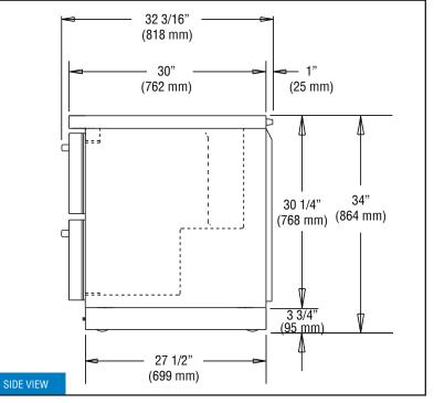
NOTE: For proper operation, the area under and in front of the cabinet must not be obstructed in any way.
