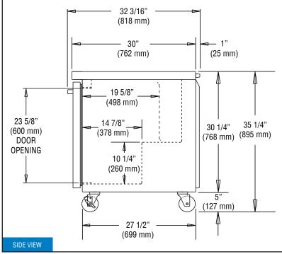
**IMPORTANT NOTE:** If the cabinet is located directly against a wall, a <u>minimum clearance of 3" is required on sides</u>, front and rear.
